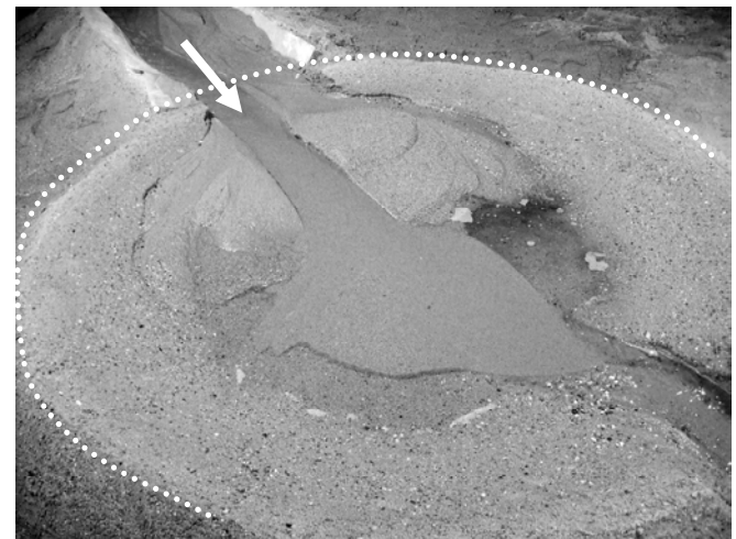
Figure 5. In contrast to Figure 4, large incised channel on the delta within the crater basin, with clearly visible terraces on each side of incised channel. Flow is from top left to bottom right. D_{50} was 0.4 mm and discharge was 0.35 \text{ m}^3/\text{s} . Flow direction indicated by white arrow, crater rim outlined with white dotted line.
