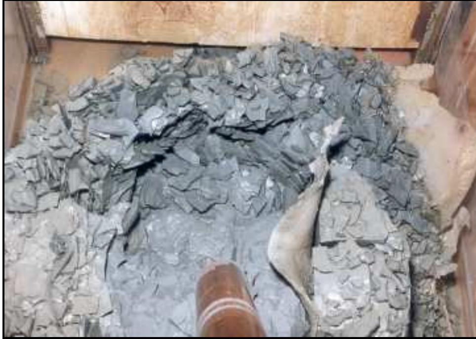
Figure 12. Scour profiles obtained with EXT1 sample with a jet velocity of 3.05 m/s
