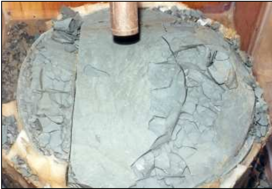
Figure 8. Surface condition after 41 hrs. of testing with a jet velocity of 2.44 m/s (EXT1)
