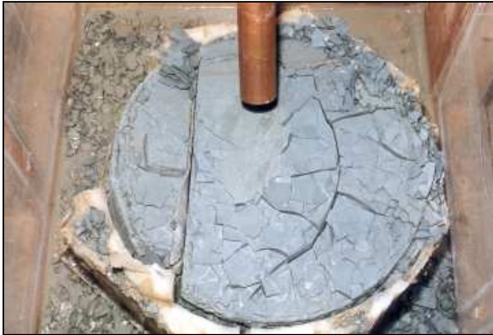
Figure 9. Surface condition after 38.5 hrs. of testing with a jet velocity of 3.05 m/s (EXT1)
