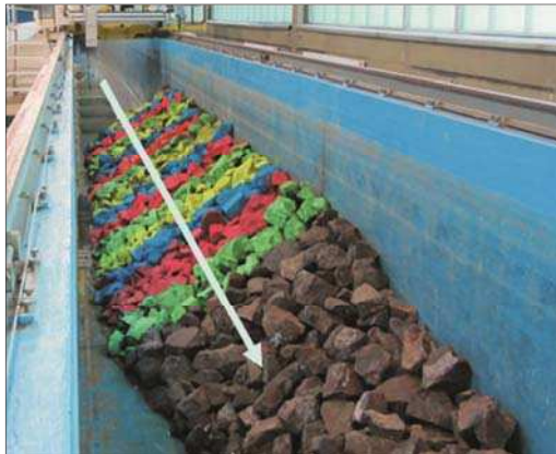
FIGURE 3. Model tests: hydraulic flume and rip-rap section with direction of overflow parallel to the slope.
