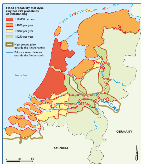
Figure 1: Safety standards as per current law (1995, Law on Water Defences), Note: these standards refer to a 90% probability that the dike rings should be able to withstand a 1 in x probability of the design water level (see Box 1 for more information)
