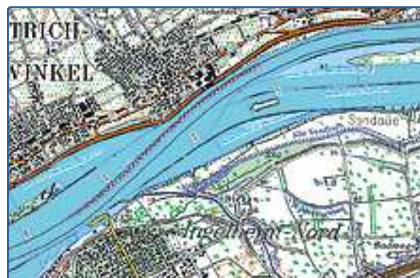
Figure 2: Test section of the trial voyages; red: narrowed fairway section; arrow: cross current from Große Gieß into Kleine Gieß
