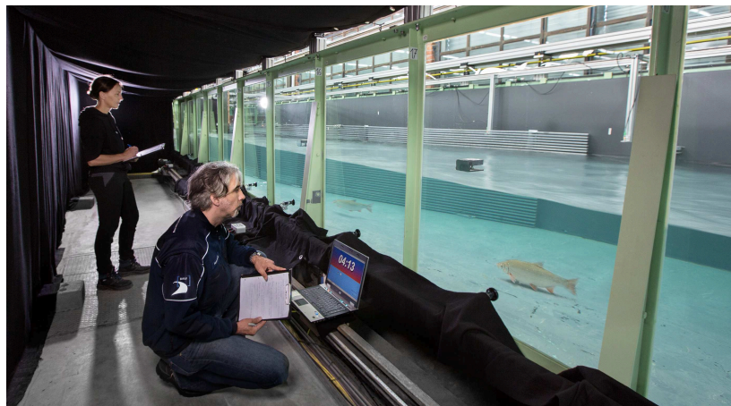
Figure 2.7: The ethohydraulic flume as seen from the observation area on the flume right, encased by black curtains. Water flowing from left to right, fish moving from right to left.
