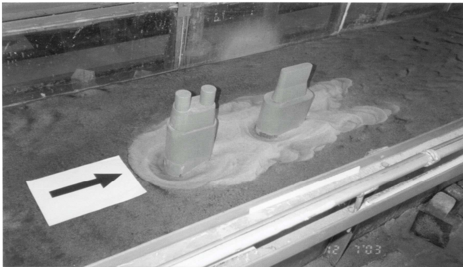
Photograph 2 - Scour and deposition pattern around the piers of the existing and proposed bridges for L/b=4.0
