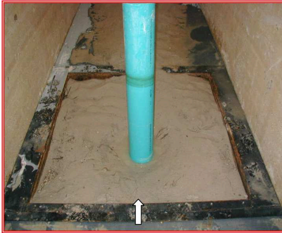
FIG 5 Scour Hole Geometry for Flume Test 1
