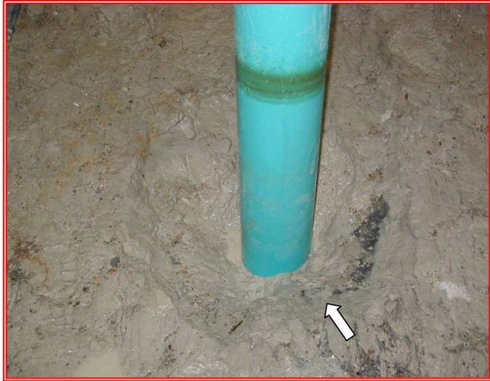
FIG 11 Scour Hole Geometry for Test 3
