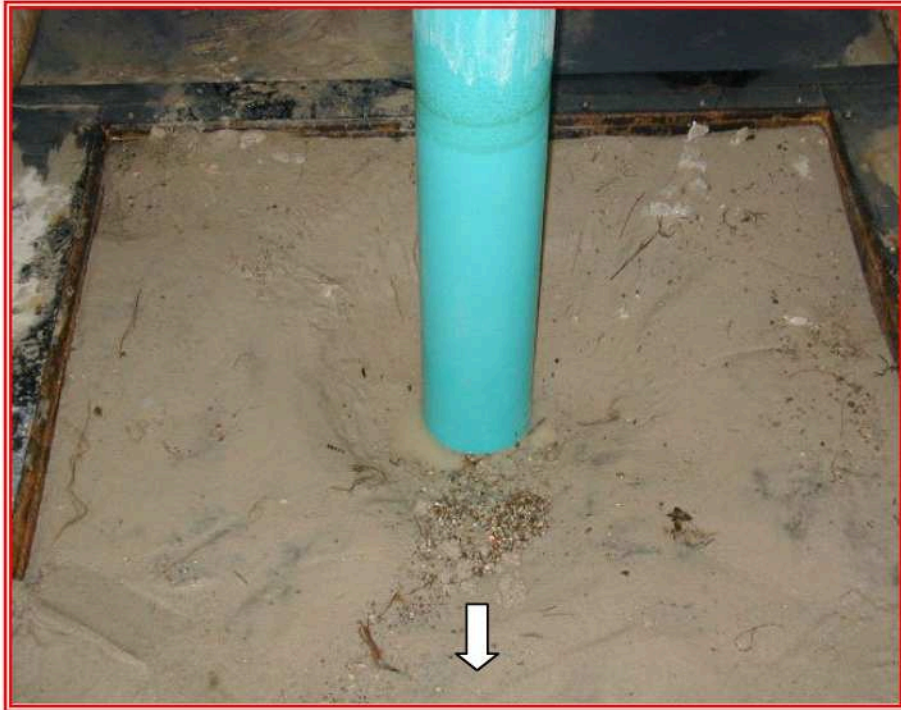
FIG 8 Back View of Scour Hole for Test 2
