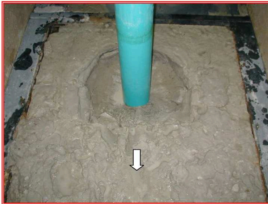
FIG 18 Back View: Scour Hole Geometry for Test 6
