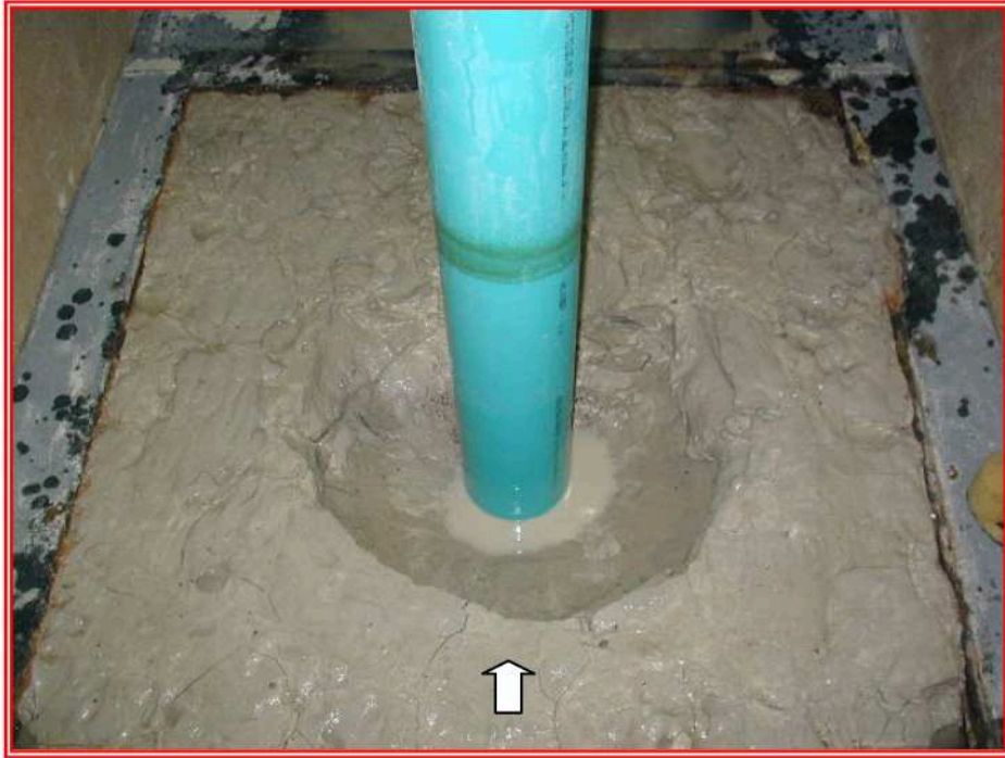
FIG 19 Front View: Scour Hole Geometry for Test 6
