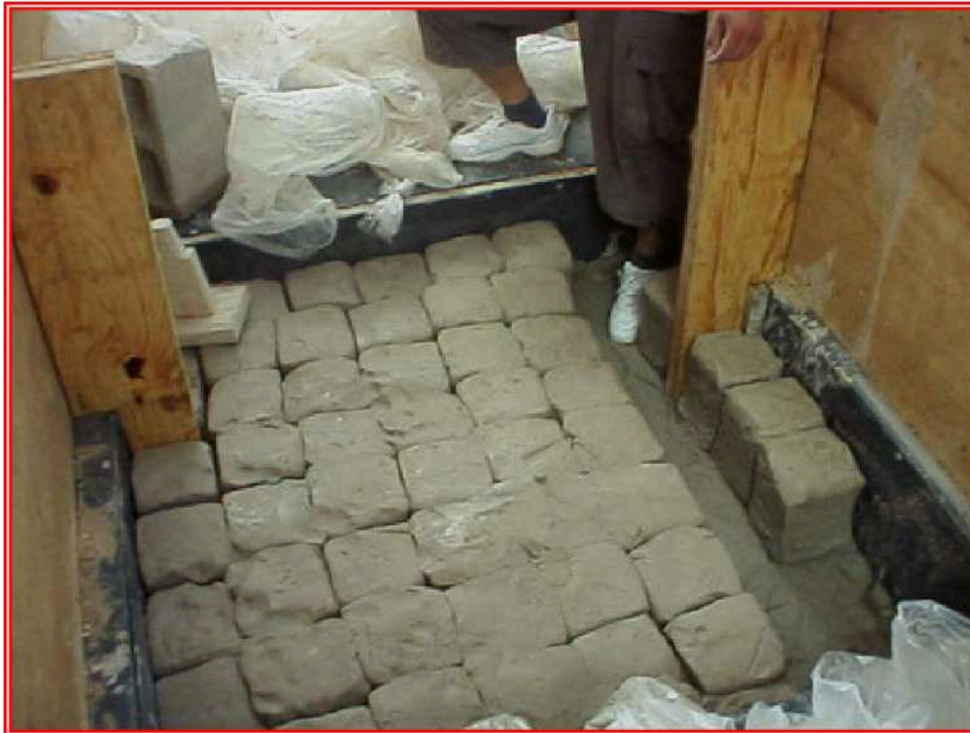
FIG 3 Preparation of the Clay Soil Tank
