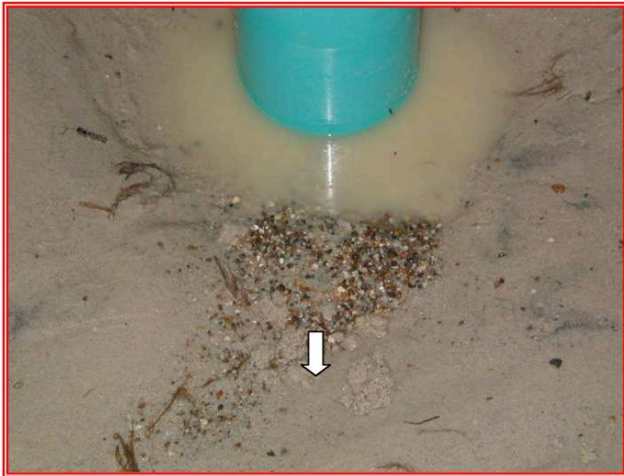
FIG 9 Coarse Particle Deposition in Test 2
