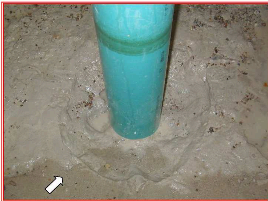
FIG 16 Scour Hole Geometry for Test 5
