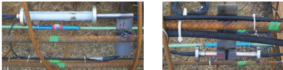
Figure 1: EFPI sensor (left) and FBG sensor (right).
