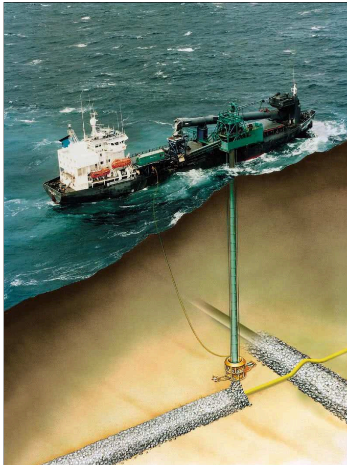
Fig. 5 – Flexible Fall Pipe Vessel “ Trollnes ”
