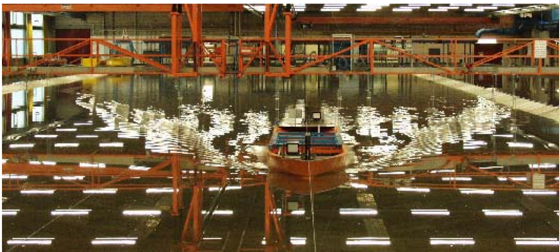
Figure 5: System test for a MEGA-JUMBO vessel underway in laterally bounded shallow water at about v_{S,MODEL} = 1.0 m/s ( v_{S,FIELD} = 12.5 kn; trapezoidal profile n = 15 ; n_T = 10 / 20 )
