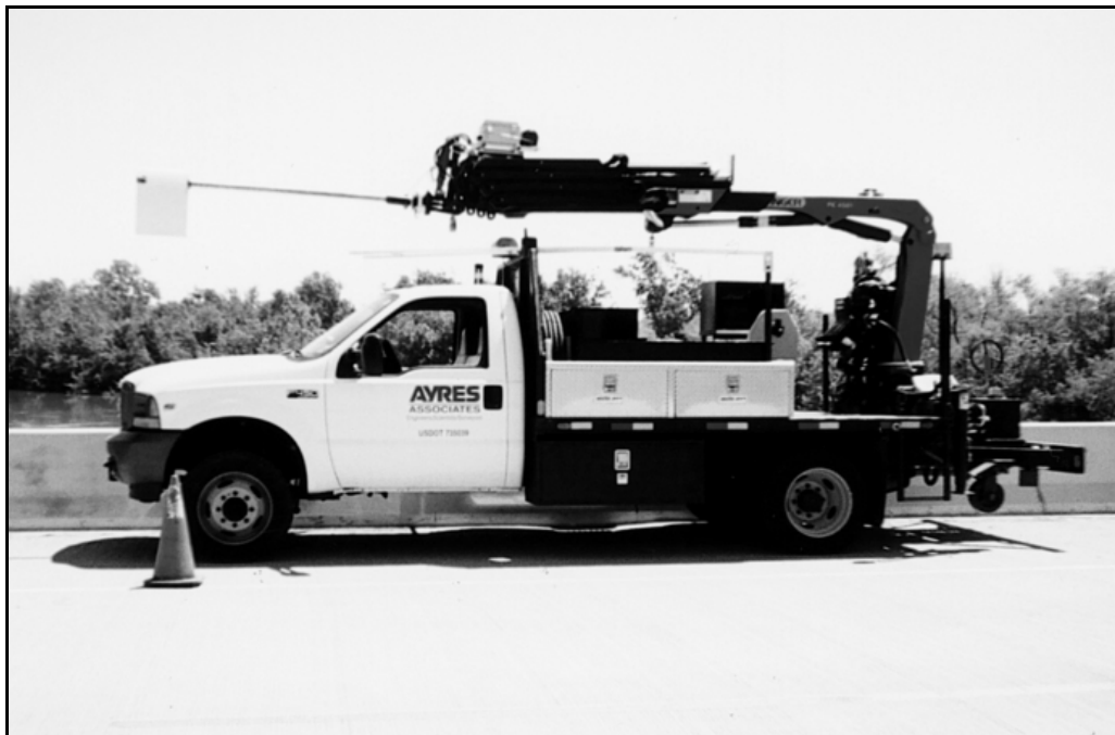
Figure 3. Completed articulated arm truck.
