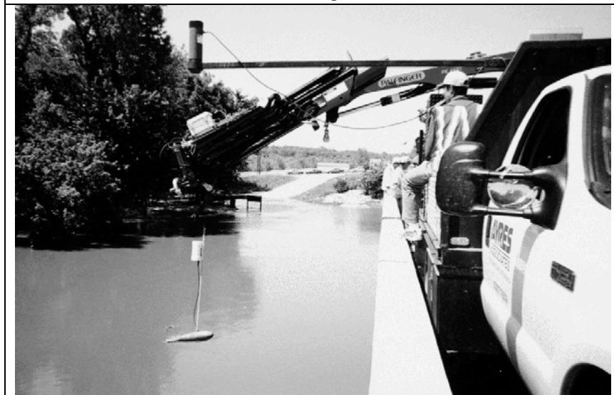
Figure 7. Wireless sonar in a sounding weight.
