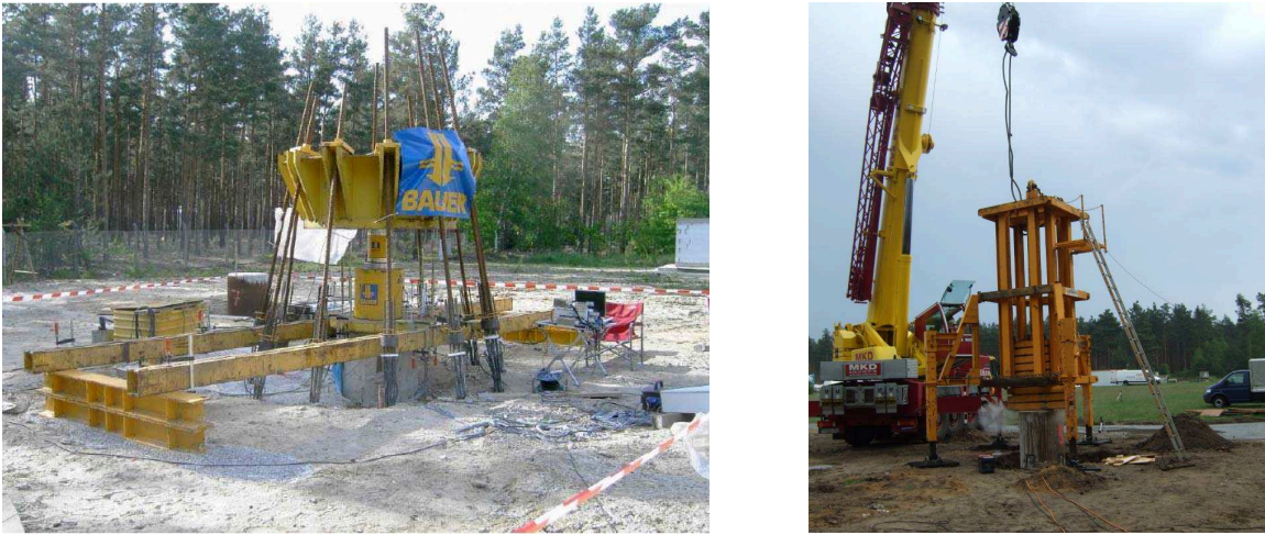
Figure 6: Static and dynamic load test setup at BAM-TTS.
