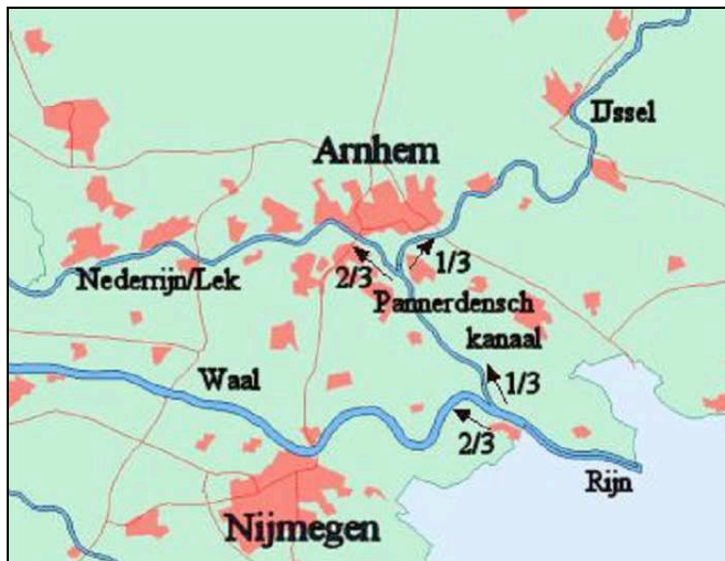
Figure 4: The Rhine branches in the Netherlands. At the bifurcation points estimates of the discharge distribution are given.
