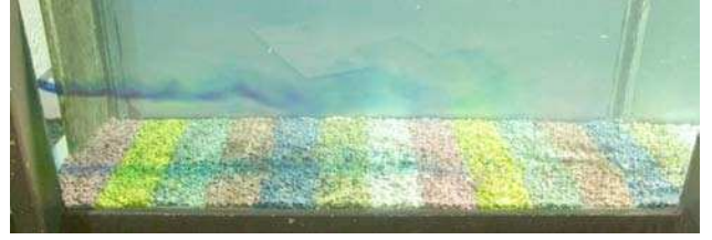
Figure 3. Experiment: flow through square opening in a vertical plate; the jet expands above the granular bed
