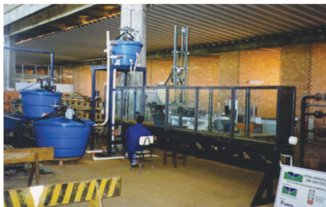
Figure 4.1. Flume for tests on silt fences (Farias 2005).
