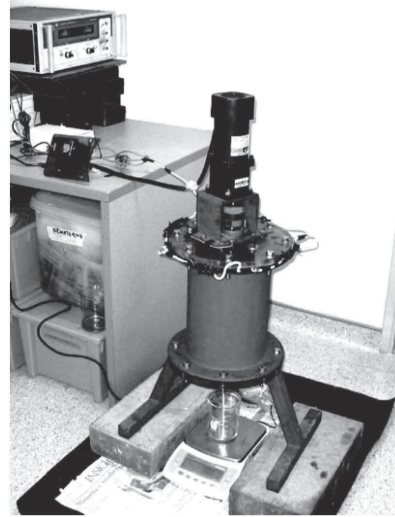
Figure 8.5. Laboratory dewatering model based on EO.
