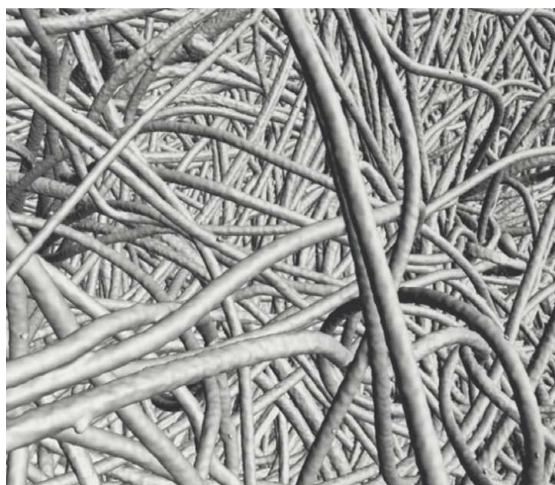
Fig. 3: View via computed tomography of a needle-punched nonwoven geotextile
