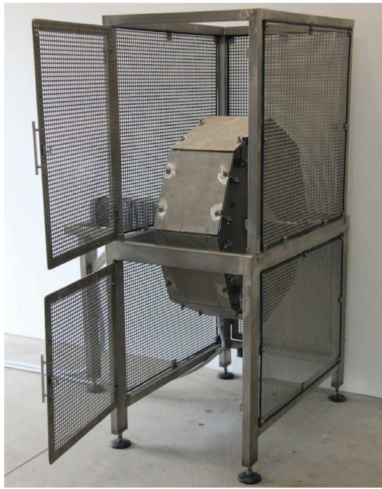
Fig. 5: Drum device for examining the abrasion resistance of geotextiles
