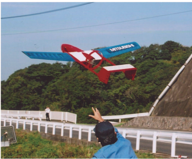
Fig.2. Takeoff of the small UAV
