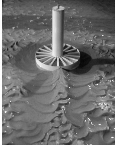
Figure 3 Result of scour test with current (Test 2)
