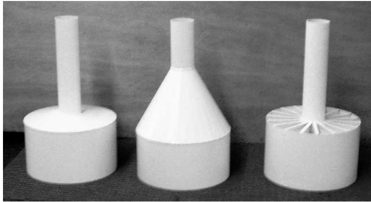
Figure 1 Foundation models used in testing – L-R: concrete-conical-girder
