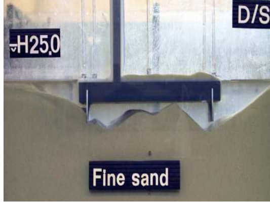
Figure 8. Final situation after complete failure
