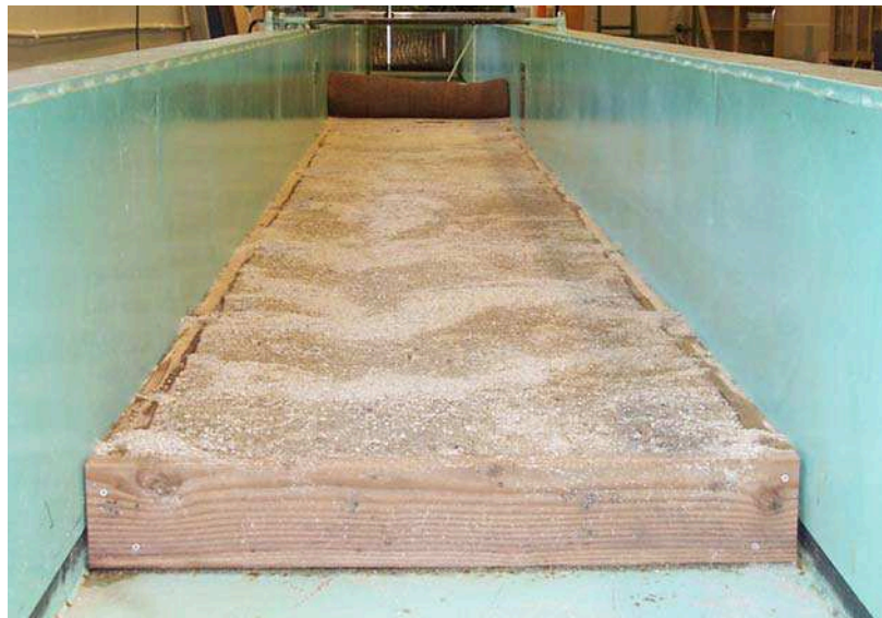
Figure 8. Soil Test Section within Flume
