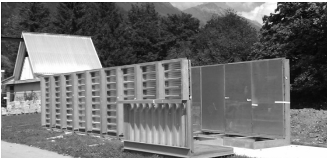
Figure 8. Modular cell concept, formed Styrofoam cubes build a natural river surface structure
