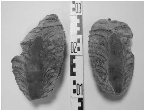
Fig. 3: The inner parts of a freeze-core. In this area, the sediment's natural structure is changed by probing.
