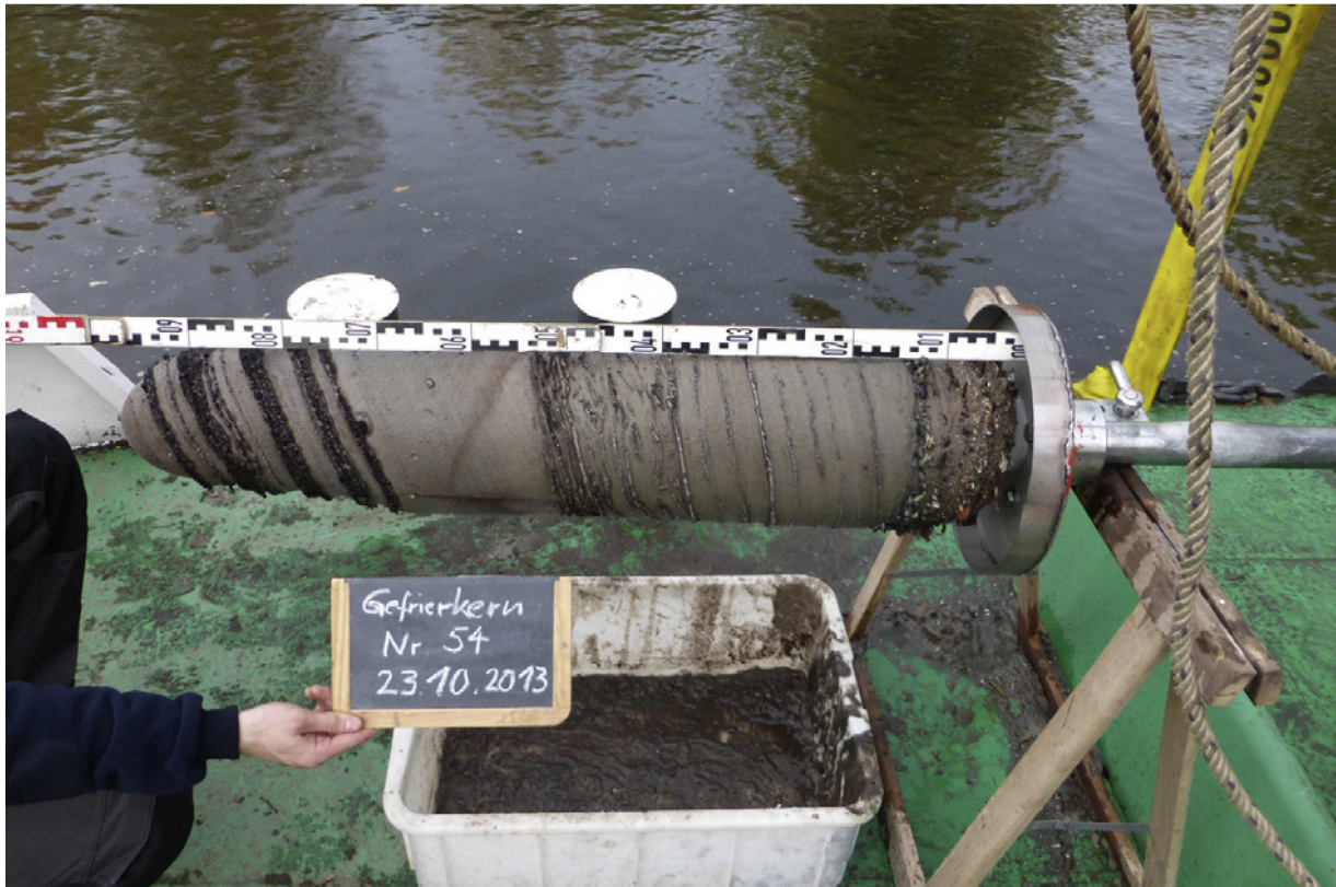
Fig. 6: Freeze-core taken from the river bed of the Sacrow-Paretz channel; sediment stratification visible.
