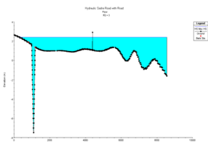
Figure (6).Profile of water surface at conditions of maximum floodtide and floodwater, in section 3
