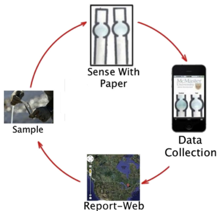
Figure 15. Concept of water quality evaluation using paper-based colorimetric sensors and a smartphone. Reprinted from Water Research, Vol. 70, Clemence Sicard, Chad Glen, Brandon Aubie, Dan Wallace, Sana Jahanshahi-Anbuhi, Kevin Pennings, Glen T. Daigger, Robert Pelton, John D. Brennan, Carlos D.M. Filipe, Tools for water quality monitoring and mapping using paper-based sensors and cell phones, Pages 360–369, Copyright (2015), with permission from Elsevier.
