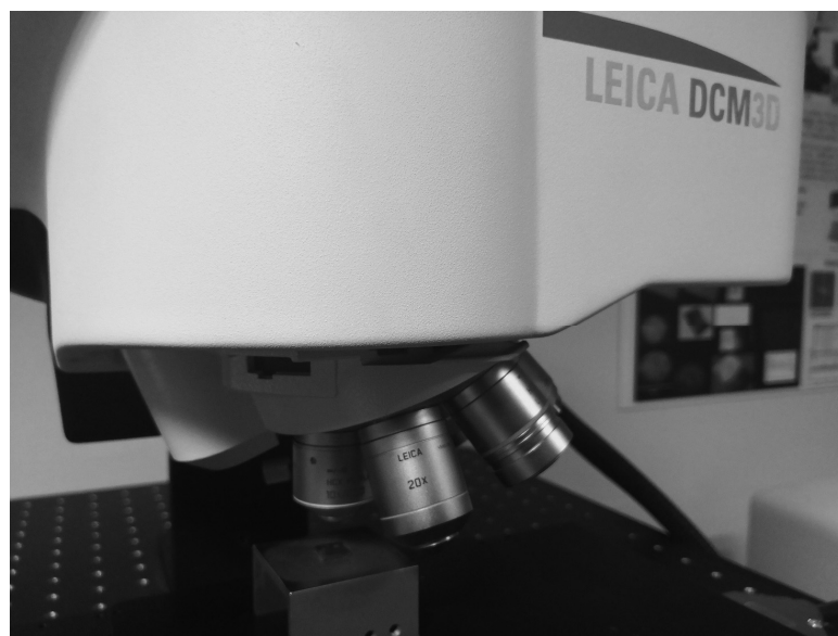
Figure 6. The sample during the profilometer analysis (MoO 3 -01 (sample #1) and MoO 3 -02 (sample #2) films on copper).
