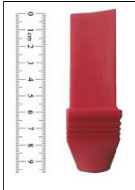
Figure 3. Prototype of the printed ABS blade.
