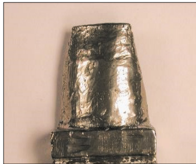
Figure 9. Barrel Finished Blade.
