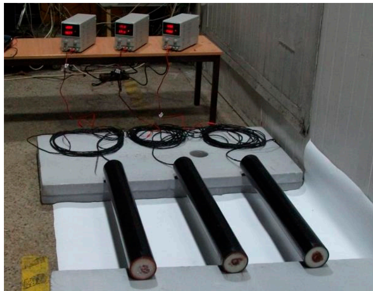
Figure 4. Electric heater during the tests.
