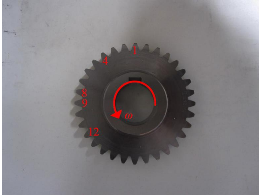
Figure 4. Numbering of the pitted teeth (4,8,9,12) of the pinion. Tooth 1 as reference.
