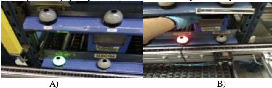
Figure 2. Diodes to inform about the selection of parts. A) Green LED indicating the order of assembly of the parts, (B) Red LED indicating incorrect part selection
