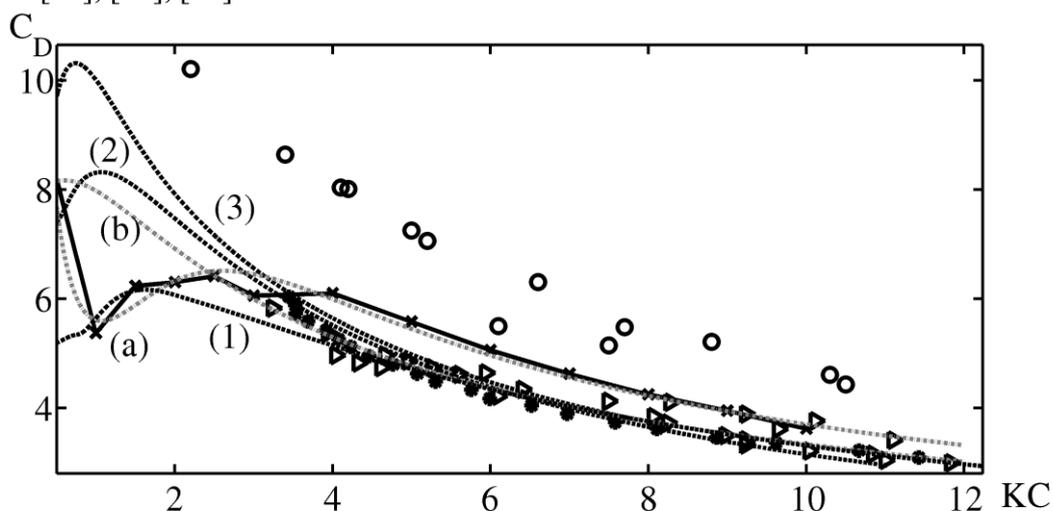
**Figure 2:** Drag coefficient  $C_D$  vs. dimensionless parameter  $KC$ . Black dotted lines 1, 2, 3 represent experimental results and solid line with cross-shaped markers represent the numerical results of the present study. Gray dotted lines a, b illustrate experimental results of [10]. Triangle markers correspond to experimental data of [13], black circles correspond to experimental data of [14] and white circles correspond to experimental data of [15].
