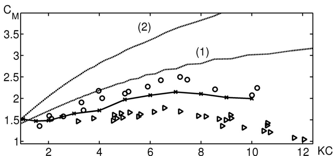
**Figure 3:** Added mass coefficient  $C_M$  vs. dimensionless parameter  $KC$ . Black dotted lines 1, 2 represent experimental results and solid line with cross-shaped markers represent the numerical results of the present study. Triangle markers correspond to experimental data of [13] and white circles correspond to experimental data of [15].
