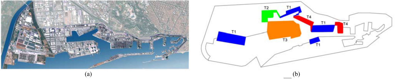
Fig. 2. Layout of the port of Barcelona. (a) Orthophotography (obtained from [48]). (b) Port terminals (authors' composition). T1 = terminal for containers and multipurpose ships; T2 = terminal for car carriers; T3 = terminal for LNG carriers and tankers; and T4 = terminal for bulk carriers.
