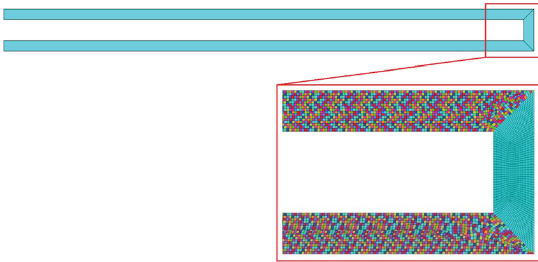
Figure 5: Elements of the FGM microactuator in ANSYS, the first and third beam are made of FGM, the second beam has constant material properties
