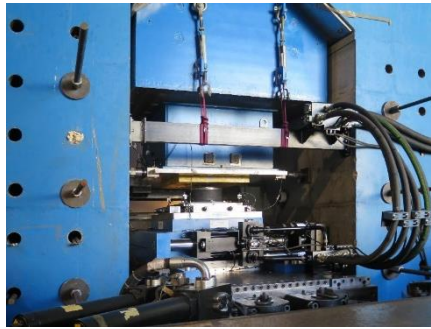
Figure 8: Bearing Testing System (BTS).
