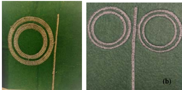
Fig.1. (a) Geometrical sketch of the proposed e-textile single and double textile DRR antenna. b) Embroidered prototypes on felt fabric.
