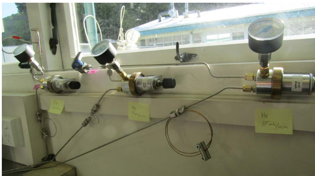
Figure 3.3 Porter regulators to provide flow control for RRL RP gas delivery system. Different resistances are introduced downstream of each regulator so the appropriate flow can be delivered. With gas flow opened via in-line valves (green for oxygen, blue for helium), the black bonnet on each regulator is turned until the required pressure is shown on the gauge. A gauge of the dual stage regulator for the helium cylinder is visible through the window.
