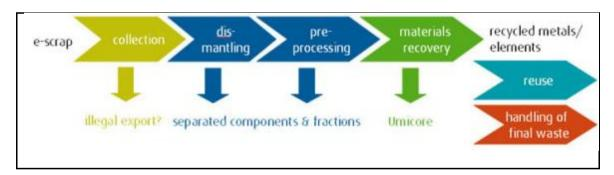
Figure 15: Typical recovery and recycling chain for WEFE<sup>68</sup>
