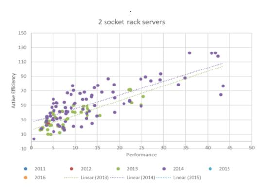
Figure 12: Relationship between performance (transactions/second) and active efficiency for two-socket servers (transactions/Joule) (higher is more efficient)<sup>38</sup>
