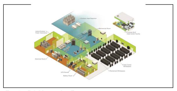
Figure 1: Typical data centre layout<sup>11</sup>
