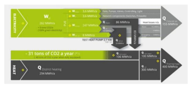
Figure 17: Example energy flow chart for a data centre in Dresden, Germany Source: Cloud & Heat (2017)
