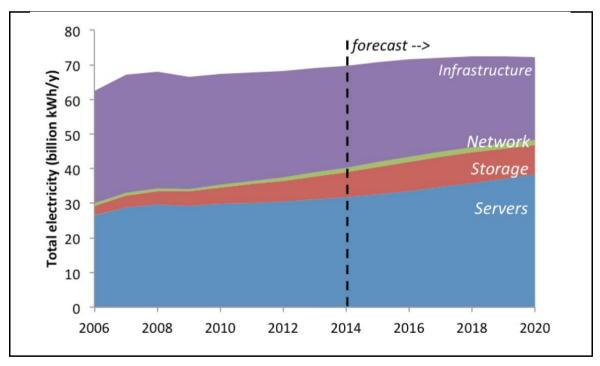
Figure 11: Total electricity consumption by technology type in a data centre<sup>37</sup>
