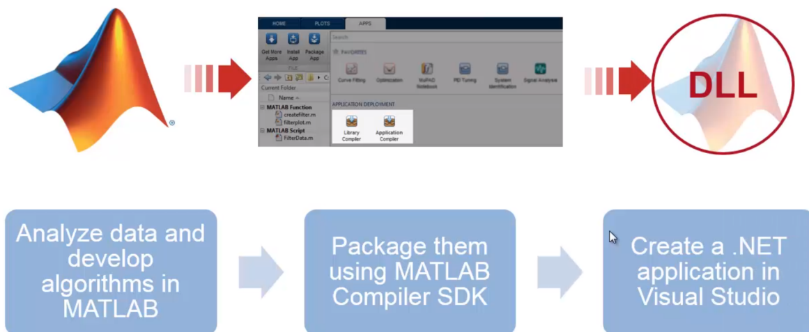
Figure 21. The process needed to import the MATLAB data in the .NET application
