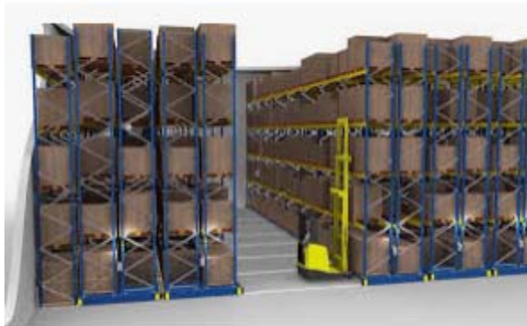
Figure 6. Mobile racking (Jungheinrich, 2015)
