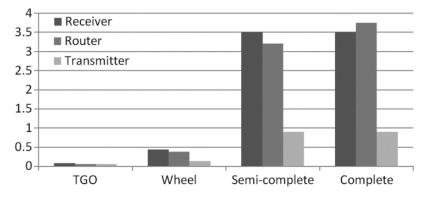
Fig. 3 — Comparison of Power Consumption of TGO Mesh with other meshes
