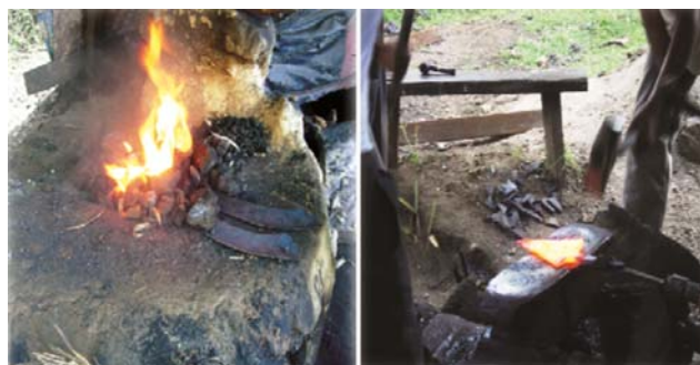
Fig. 2 — The iron-rod burned till-red hot
