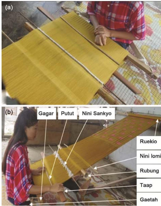
Fig. 2 (a) — Top view of Rubung ruekia , (b) Different components of Rubung ruekia
