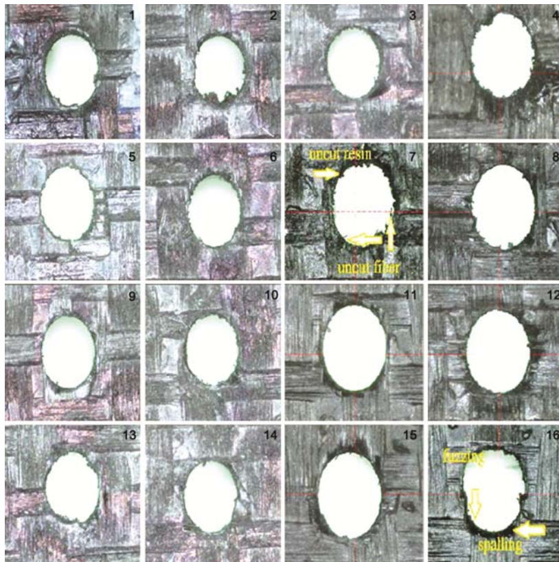
Fig. 9 — Machined hole at the exit side in MD.
