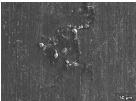
Fig. 12 — SEM micrograph of type 1 steel plasma coated under condition 1 (63% Ar).
