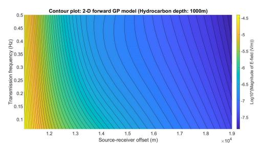
**Figure 6.** Contour plot of the 2D forward GP model. EM responses versus source-receiver separation distance for all tried and untried transmission frequencies (0.0625–0.5 Hz) at overburden thickness of 1000 m.
