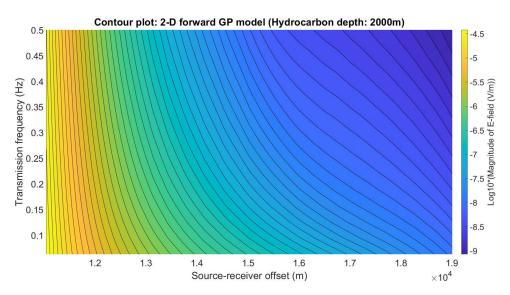
**Figure 7.** Contour plot of the 2D forward GP model. EM responses versus source-receiver separation distance for all tried and untried transmission frequencies (0.0625–0.5 Hz) at overburden thickness of 2000 m.
