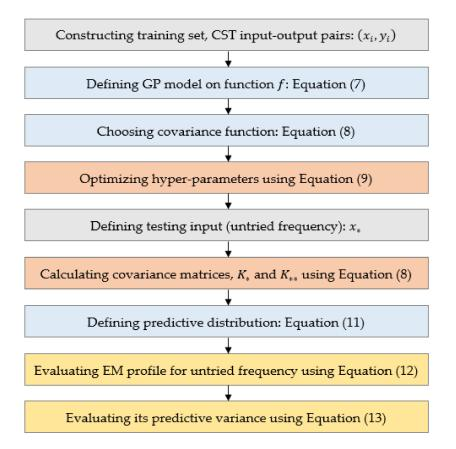
**Figure 2.** Simplified methodological flow of GP regression modelling in SBL data generated through the CST software.
