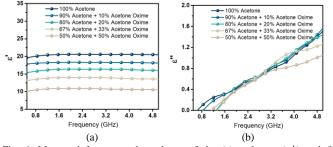
Fig. 4. Measured frequency dependence of the (a) real part ( $\varepsilon'$ ) and (b) imaginary part ( $\varepsilon''$ ) of the relative complex permittivity of acetone and its mixtures with acetone oxime at different concentrations.
