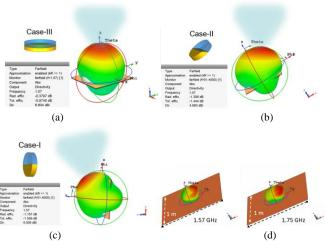
Fig. 8. 3D radiation patterns and gains of the proposed antenna at 1.57 GHz under three different cases of tilt. (a) Flat. (b)  $45^{\circ}$  tilt. (c)  $90^{\circ}$  tilt. (d) Radiation patterns at 1.57 and 1.75 GHz when the antenna is mounted on a large metal ground of 1 m  $\times$  1 m.
