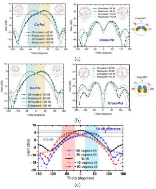
Fig. 10. Simulated and measured E-plane (YOZ-plane) radiation pattern of the proposed antenna under (a)  $+/-45^{\circ}$  tilt. (b)  $+/-90^{\circ}$  tilt. (c) Simulated E-plane radiation patterns for +/-45 and  $+/-90^{\circ}$  physical tilts of the antenna.
