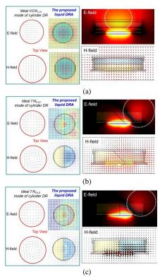
Fig. 9. Simulated contour plots of E-fields and H-fields of the antenna under the three aforementioned cases. (a) Case-III. (b) Case-II and Case-IV. (c) Case-I and Case-V. The field distributions of the ideal  $TM_{01\delta}^z$  and  $HEM_{11\delta}$  modes for cylinder DR are presented for comparison (taken from [18]).
