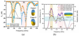
Fig. 7. (a) Simulated and measured reflection coefficient  $(S_{11})$  of the liquid antenna under Case-I and Case-V (antenna is tilted 90°). (b) fMeasured and simulated radiation efficiency and total efficiency of the proposed liquid antenna under Case-III over the frequency band of interest.
