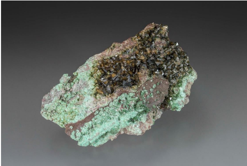
Figure 15. This specimen includes adamite – olivenite series minerals of several compositions. The pseudo-octahedral crystals at upper right (as photographed) are yellowish-brown in color, but some have a distinct pinkish blush. The mean MP_{Cu} for the brown crystals is 9.38 % (range: 0.88 – 18.04 %) while the pinkish crystals contain a mean MP_{Cu} of 1.62 % (range: 0.27 – 4.60 %). The mean cobalt content of the pinkish crystals is 0.045 wt % (see text for further details). 9.5 cm. Malcolm Southwood specimen (# MS 2016.076) and photo.
