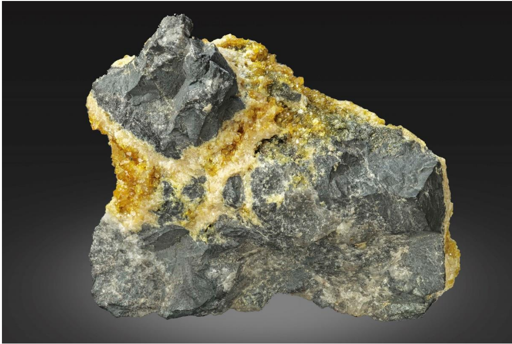
Figure 13. Long prismatic crystals of orange-yellow adamite on mineralised dolostone. The mean MP_{Cu} is 1.11 % (range: 0.02 – 3.25 %), so the adamite is close to end member composition. 10 cm. Crystal Classics specimen and photo.
