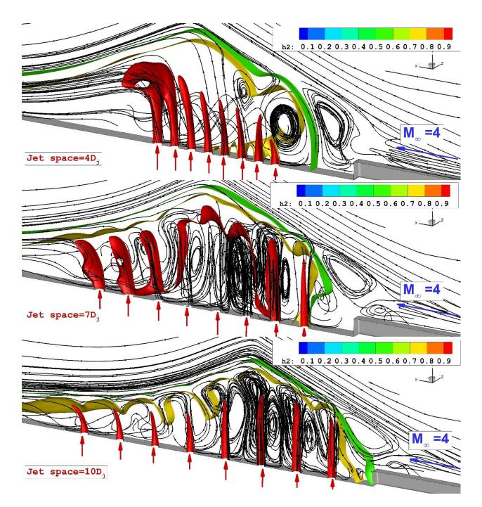
Fig. 6 comparison of the multi fuel jets with different jet spacings in presence of upstream backward step
