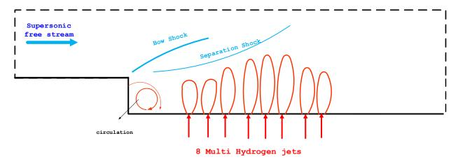
Fig.1 Schematic of backward-facing step in supersonic flow
