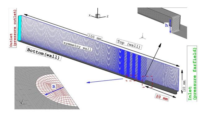
Fig. 2 size and geometry of upstream backward step
