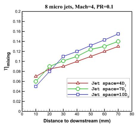
Fig. 9 Mixing efficiency for different jet space at model with upstream backward-step
