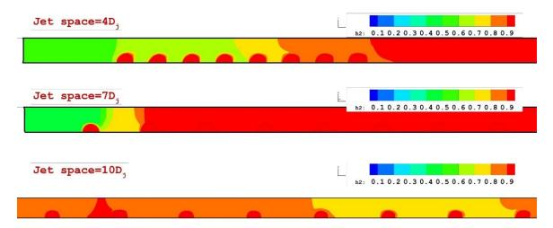
main stream interacts with a top wall in the middle of the jets, the temperature increases at the top of the jets. In the case with jet space of 10Dj, just one circulation is observed in the upstream of the first jet.
