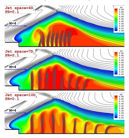
Fig. 7 temperature contour on the jet plane
