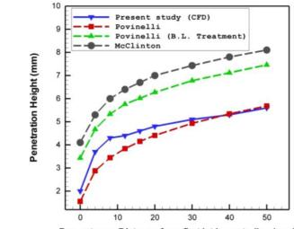
Downstream Distnace from first jet in centerline (mm)
