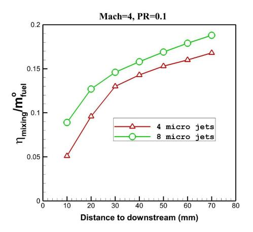
Fig. 10 comparison of the mixing ratio of 4 and 8 micro jets
