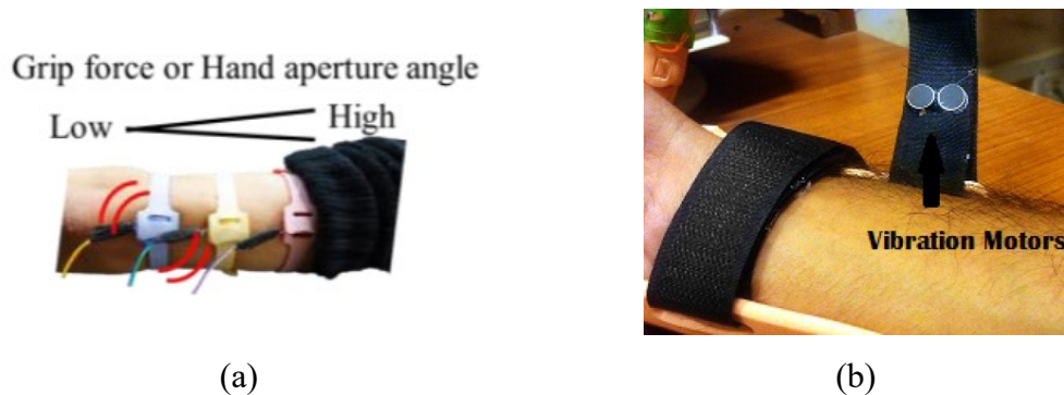
Figure 2.2 - Examples of Vibrators used in Vibrotactile feedback (a) Spatially Placed Vibrators [44] © 2016 IEEE; (b) Coin Vibration Motors [46] © 2016 IEEE.
