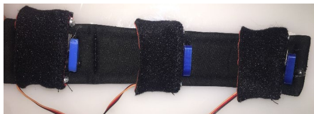
Figure 5.4 - Mechanical crank setup with three mechanical motors on leash cuff
