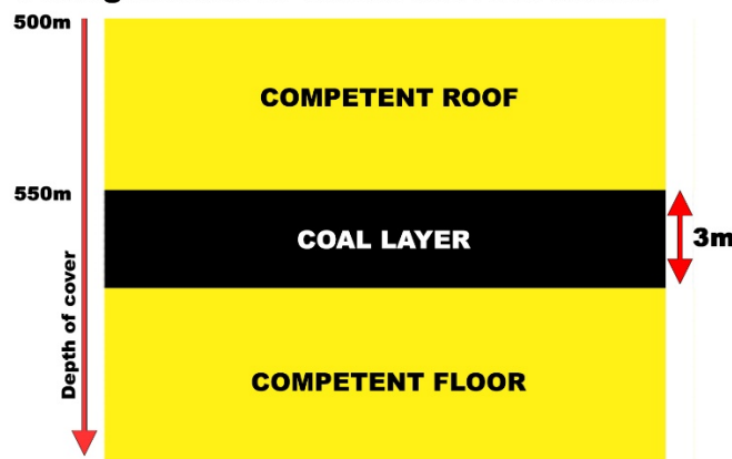
Configuration of Strata in FLAC Model
