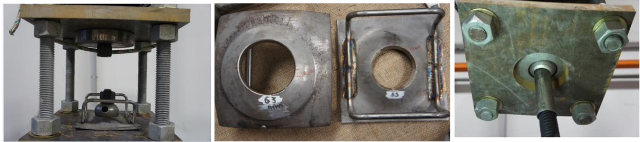
Figure 5: Dome washer plate and enlarged plate hole with the bolt spherical grout injection dome being pulled through the plate
