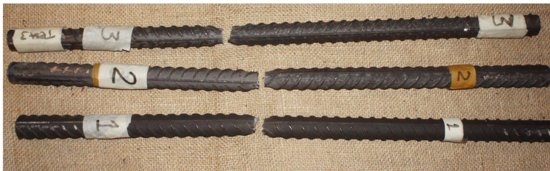
Figure 3: Pull tested rock bolts to failure, the failure points were at /near the middle of each test sample. Note the cone and cup failures of snapped bolt at the necking zones.
