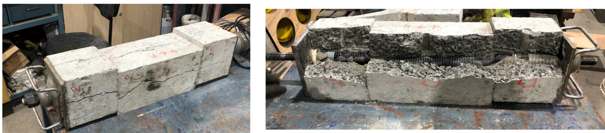
Figure 12: photos of double shear tested block and exposed grouted bolt post testing
