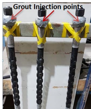
Figure 7: Sleeve grouting on to bolts
